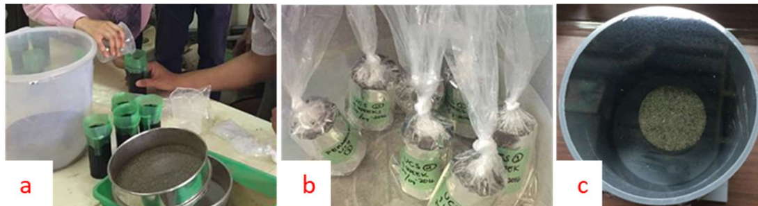
Figure 2. (a) Screening of medium well sand and sample creation (b) curing sample (c) Dutch Tank Leaching test
