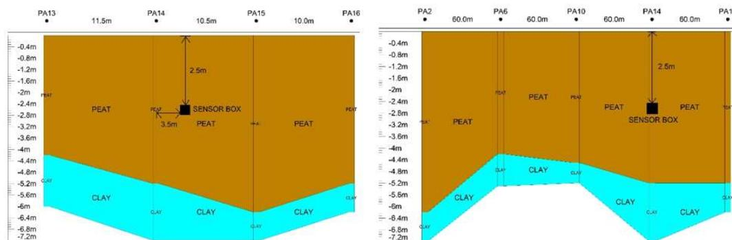
Figure 2. Soil profile: (a) cross section, (b) long section
