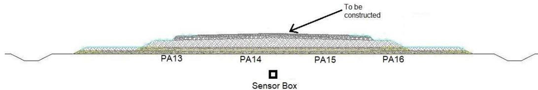
Figure 6. Road embankment and roadway to be constructed on top of peat
