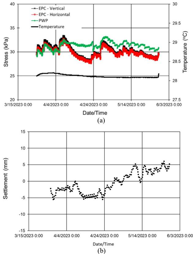
Figure 7. Current reading of sensors: (a) stress and temperature, and (b) settlement
