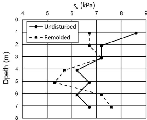
Figure 4. Undrained shear strength vs depth at PA14
