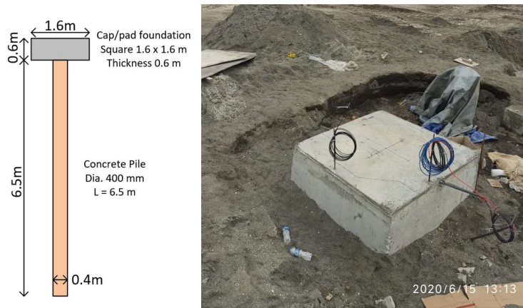
Figure 2. Geometry of the foundation (PT. GEC, 2020)
