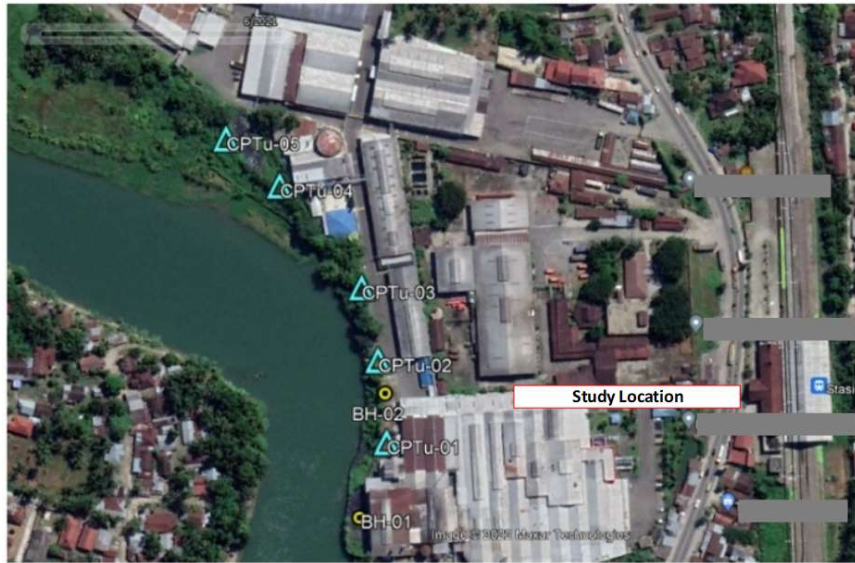
Figure 7. Latest soil investigation layout
