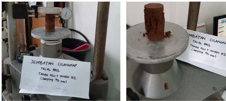
Figure 31. Unconfined compression test to the soil cement sample after soaked for 7 days
