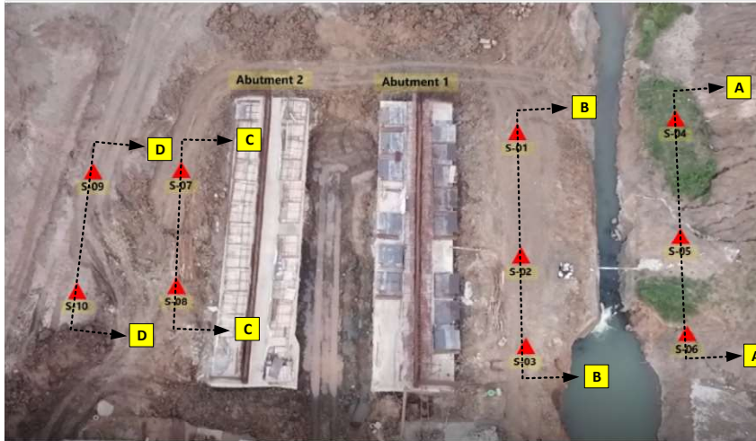
Figure 15. Layout of additional cone penetration tests location
