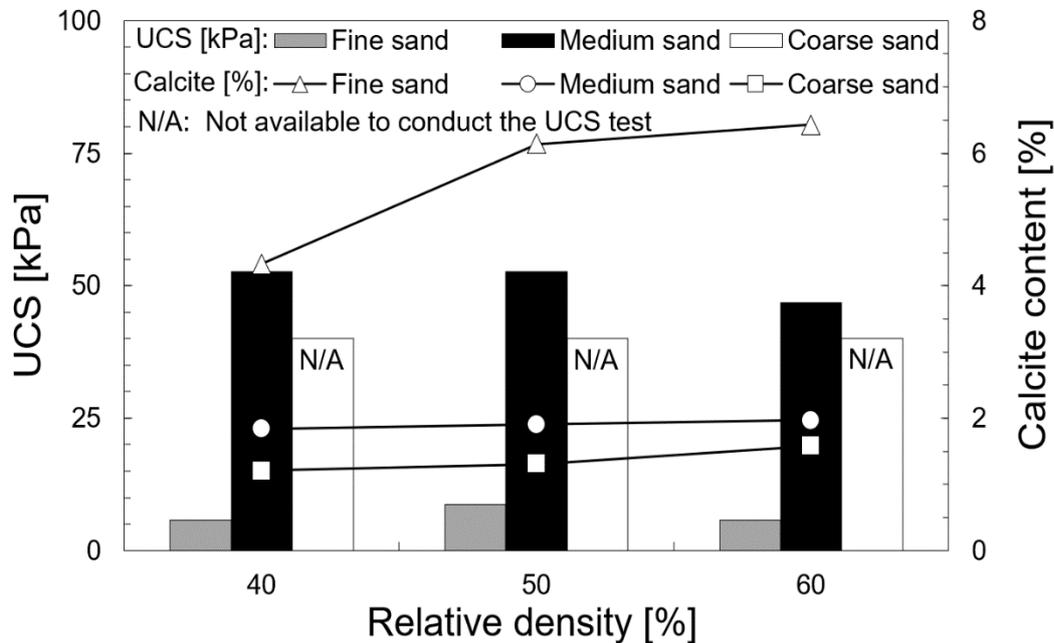
Figure 4. The UCS test and calcite content results
