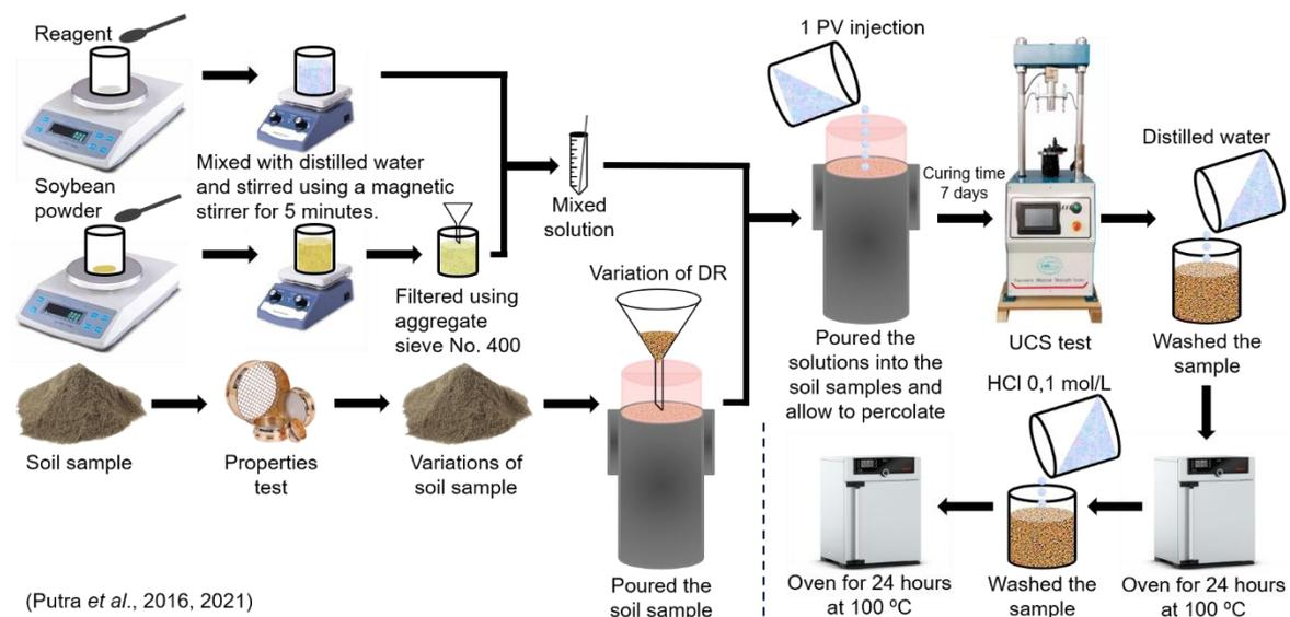
Figure 3. The procedure of soybean crude urease-calcite precipitation soil treatment method in this research (Putra *et al.*, 2016, 2021).
