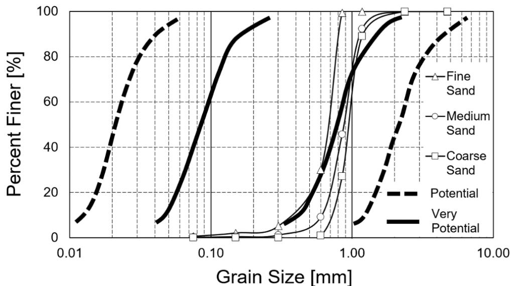
Figure 2. Soil gradation curve of fine, medium, and coarse sand. Note: potential and very potential line refers to the liquefaction potential by Tsuchida (1970).
