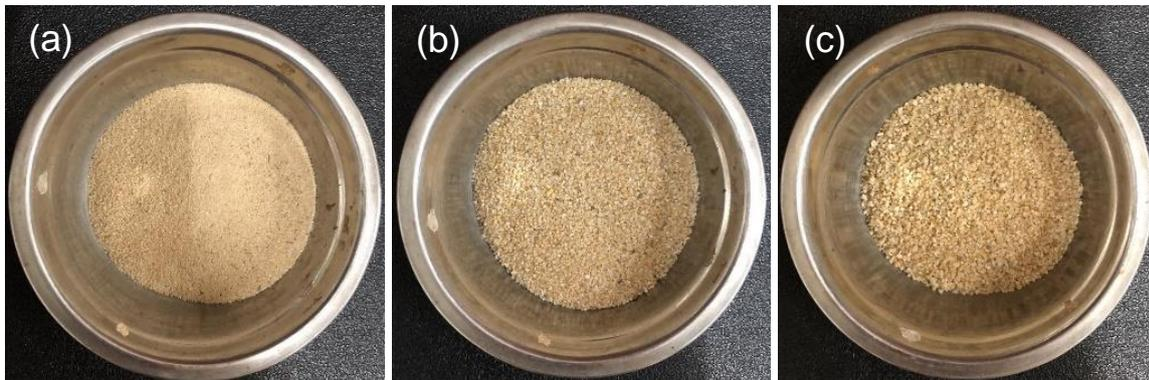
Figure 1. Sand used in this research, (a) fine sand, (b) medium sand, and (c) coarse sand.
