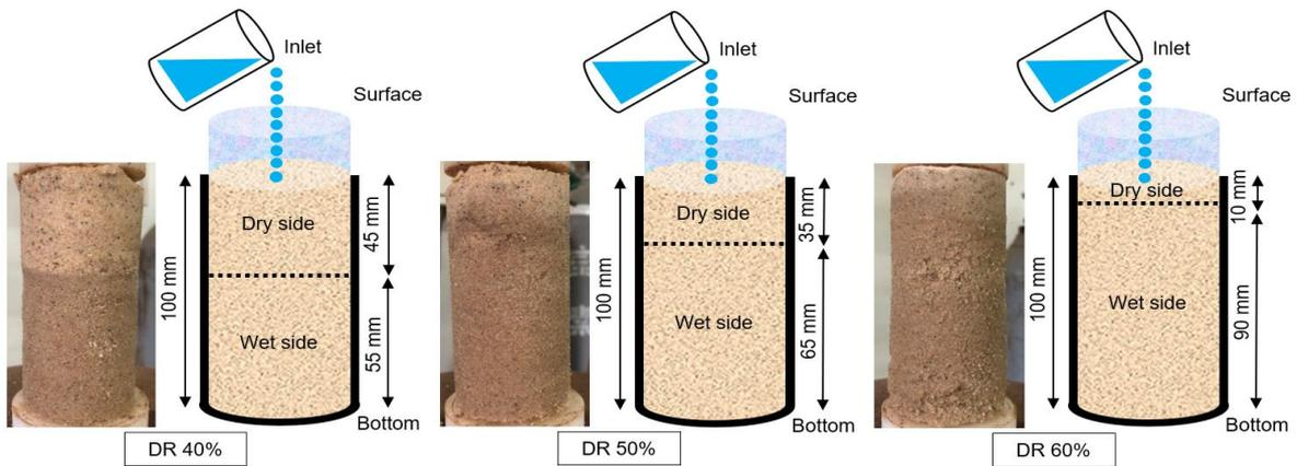
Figure 5. Fine sand in different relative densities after 7 days of curing
