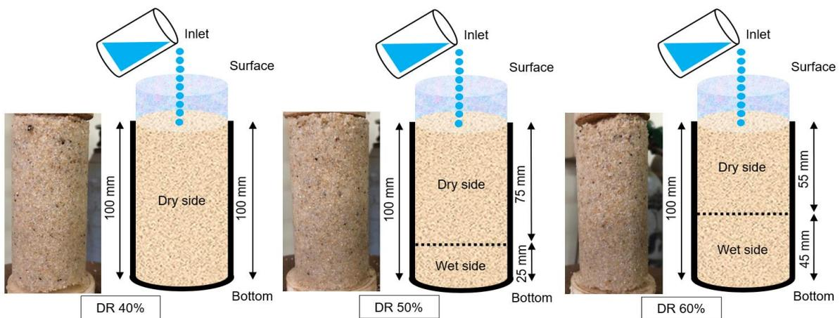
Figure 6. Medium sand in different relative densities after 7 days of curing
