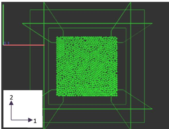
Figure 2. Particle pack using DEM in YADE (1-2 plane)
