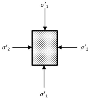
Figure 4. Principal global stress in the numerical specimen.
