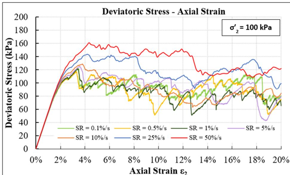
Figure 7. Deviatoric stress – axial strain curve parametric study results.
