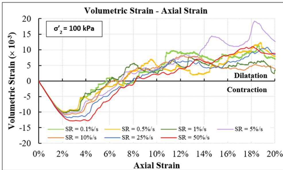
Figure 8. Volumetric strain – axial strain curve parametric study results.
