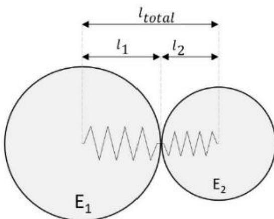
Figure 1. Normal stiffness in the contact area between particles in the Linear Elastic-Plastic contact model.
