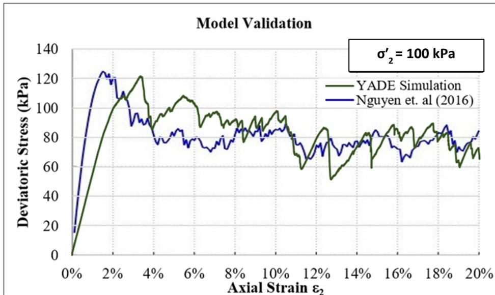
Figure 5. Deviatoric stress–axial strain from YADE simulation with strain rate value of  $1\% \text{ s}^{-1}$ : (green) this study; (blue) Nguyen et al. (2016).
