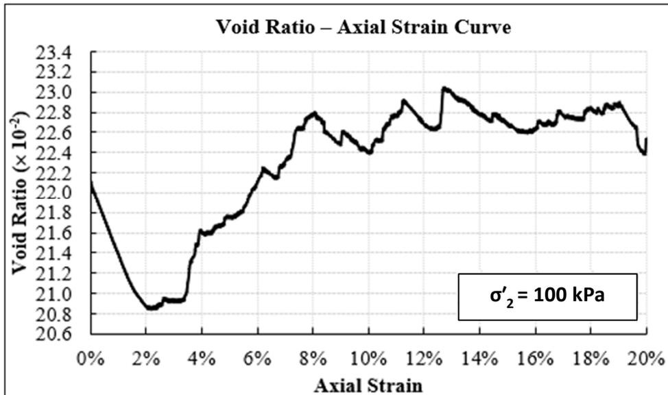
Figure 6b. Two-dimensional (2D) void ratio – axial strain from YADE simulation with strain rate value of  $1\% \text{ s}^{-1}$ .
