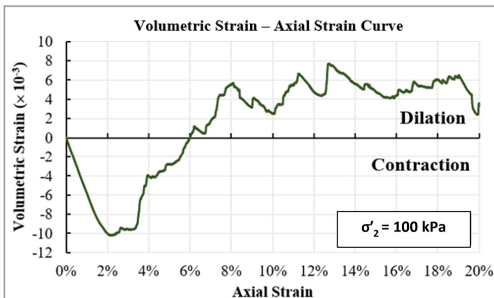
Figure 6a. Volumetric strain – axial strain from YADE simulation with strain rate value of  $1\% \text{ s}^{-1}$ .
